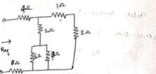
Soln:  $\Rightarrow 6\Omega$  &  $3\Omega$  resistors are in parallel.
