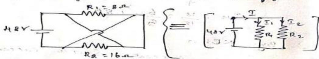
14. Find the current flowing below by using mesh analysis
