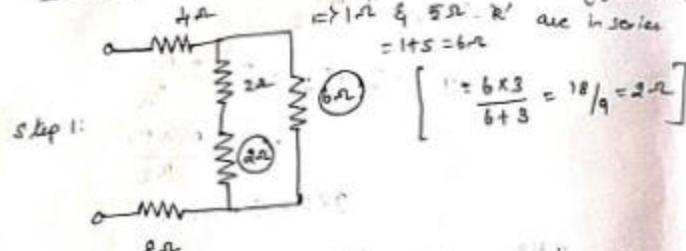
$$\Rightarrow 1\Omega \text{ & } 5\Omega - R' \text{ are in series}$$
