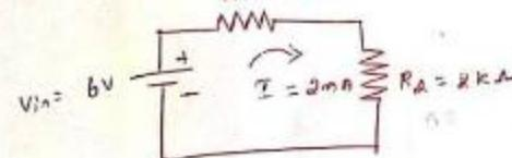
$$\begin{aligned} \text{Voltage across } R_1: V_1 &= IR_1 = 2 \times 10^{-3} \times 1 \times 10^3 \\ &= 2\text{ V} \end{aligned}$$
